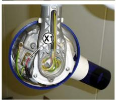
6. Check the plug contacts on the connector (X1) for damage.
