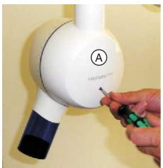
9. Attach and secure the cover (A).
