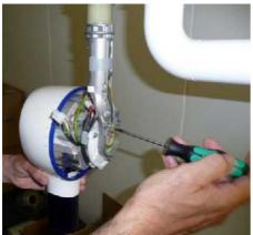
**2.** Firmly attach the X-ray tube assembly, using 3 new self-cutting screws (PM 3.5 x 16).
