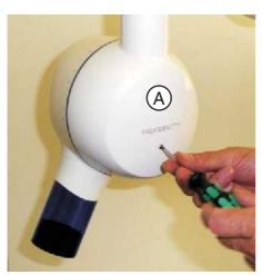
1. Unscrew and remove the cover (A).
