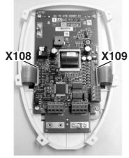
4. Unlock the foil cable sockets X108 and X109.
